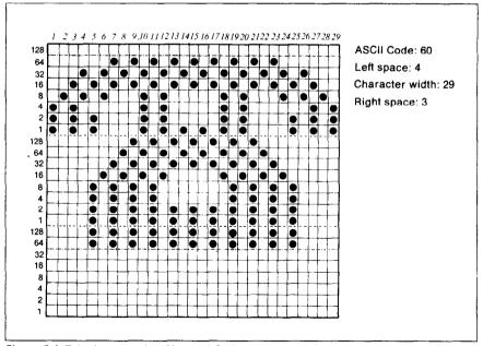
Figure C-1. Telephone symbol, Normal LQ pica
