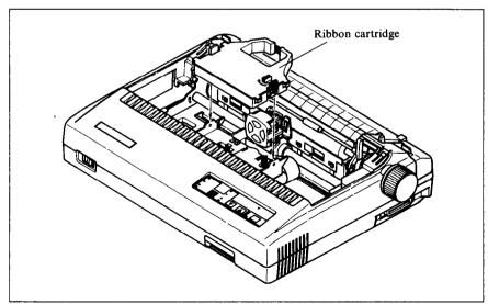
Figure 1-4. Installing the ribbon cartridge
