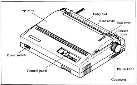
Figure 1-2. The printer's external parts
