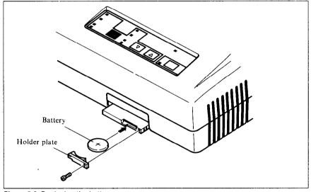
Figure 5-3. Replacing the battery
