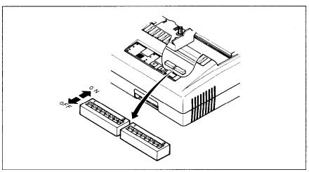
Figure 1-15. DIP switches
