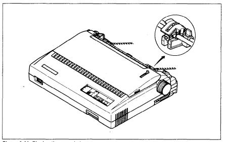
Figure 1-11. Closing the sprocket covers
