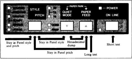
Figure 2-2. Power-up functions of control panel
