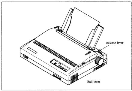
Figure 1-8. Loading a single sheet
