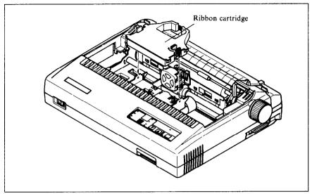
Figure 5-1. Replacing the ribbon cartridge
