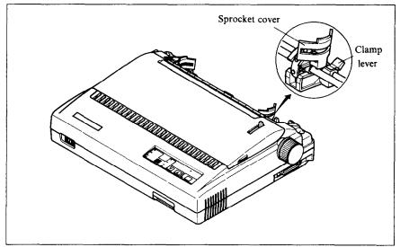
Figure 1-10. Opening the sprocket covers to expose the sprocket teeth
