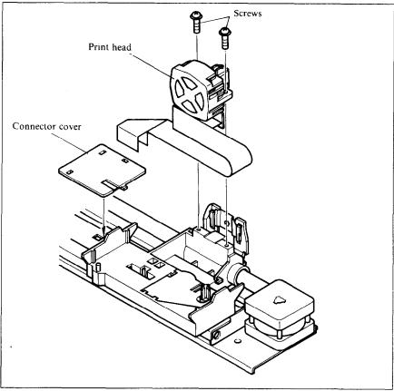
Figure 5-2. Replacing the print head
