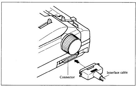
Figure 1-6. Connecting the interface cable
