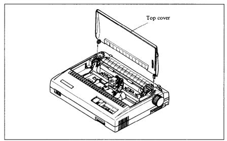
Figure 1-3. Removing the top cover
