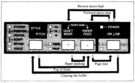
Figure 2-5. Switch combination functions of control panel
